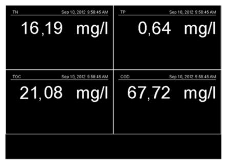
The figure gives an example of the QuickTOC<sub>NPO</sub>'s display showing all four parameters while monitoring the effluent stream of a waste water treatment plant.
