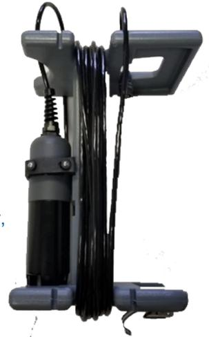
the desired test location. The rugged design was built specifically for the rigors encountered by field instrumentation. The PortaCaddie was designed to offer a level of protection to the meter, sensor, and cable.
