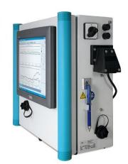
Flurometric determination using the AlgaeOnlineAnalyser is highly sensitive due to the use of a low-noise photo-multiplier.
