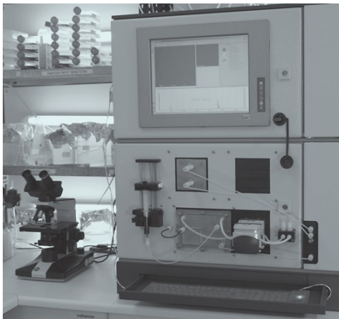
Daphnia Toximeter II in the lab
