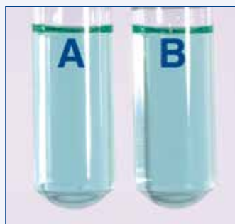
2 tubes (A / B) with the same COD concentration Deviations up to 30 % are possible.
