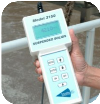
A portable unit in use in a waste water facility
