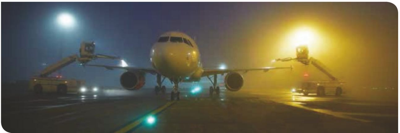
Aircraft de-icing: Existing or forming frost is removed by de-icing fluids directly before the plane starts. The de-icers in use (acetates, glycols or formates) are mixed with water and additives.
