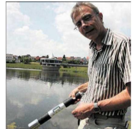
Water check: environmental engineer Gründel determines excellent water quality and an adherence to guidelines in Lake Twiste with an AlgaeTorch.
