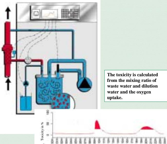
As with the BIOX-1010, the microbes grow on the inner surface of small hollow cylinders. They take up the dissolved oxygen almost completely.
