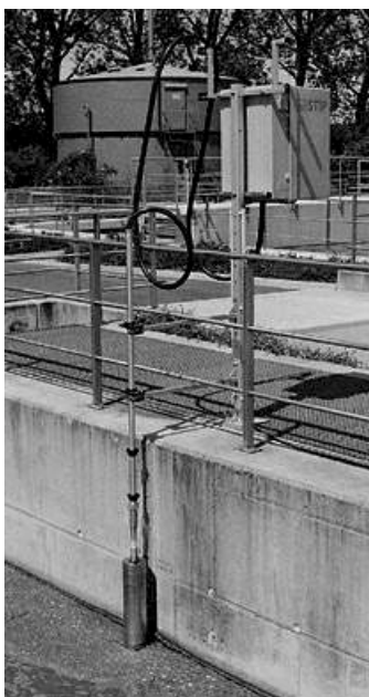
FIG 4 Isco-STIP process buoy for In-situ Ammonia-N measurement
