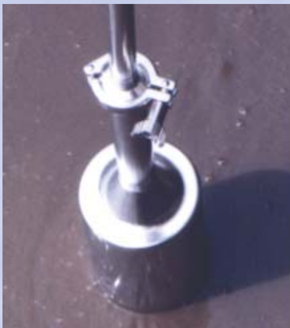
Fig. 1: STIP-scan in an aeration tank of a wastewater treatment plant
