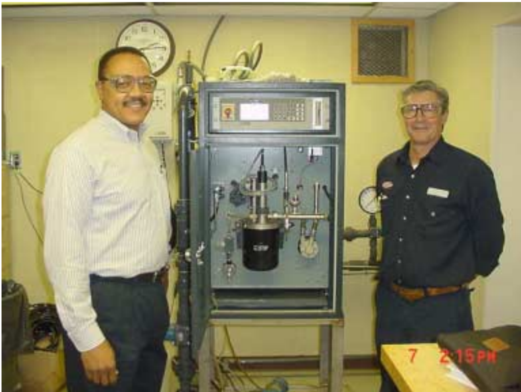
{Caption} Mr. Bob Cousar (left) and Mr. Frank Distefano (right) with Isco / Stip BIOX 1010 continuous on-line BOD Analyzer
