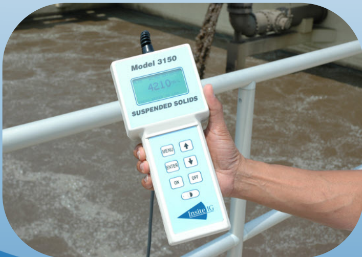
A portable unit in use in a wastewater facility
