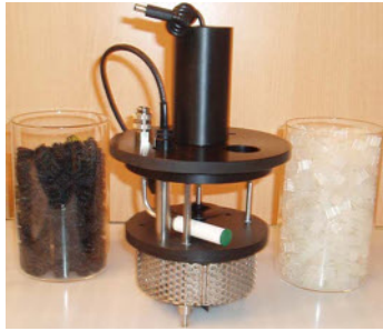
Optional adaptation for testing biomass carriers
