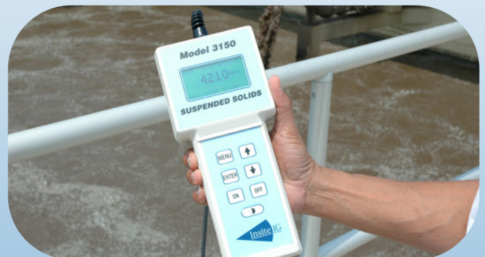
A portable unit in use in a wastewater facility
