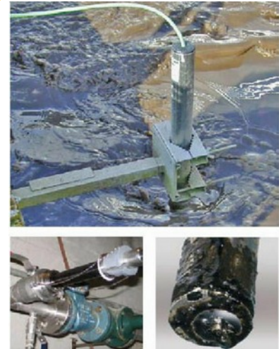
In tank mounting, "hot tap pipe mount", mechanical optics wiper
