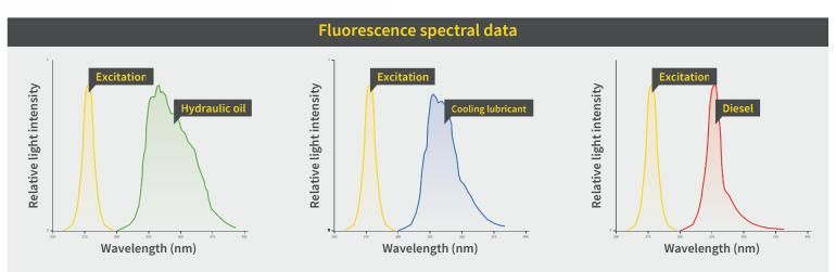
There is no universal fluorescence spectrum for all oils. Rather, the spectrum depends on the composition of the oil. Refined oils consist mainly of aromatic hydrocarbons, which in solution in water are often indicated in the BTEX collection parameter. The graph shows examples for typical fluorescence spectra of some refined oils. The BlueTrace oil in water sensor is suitable for the measurement of refined oils, BTEX and aromatic hydrocarbons.
