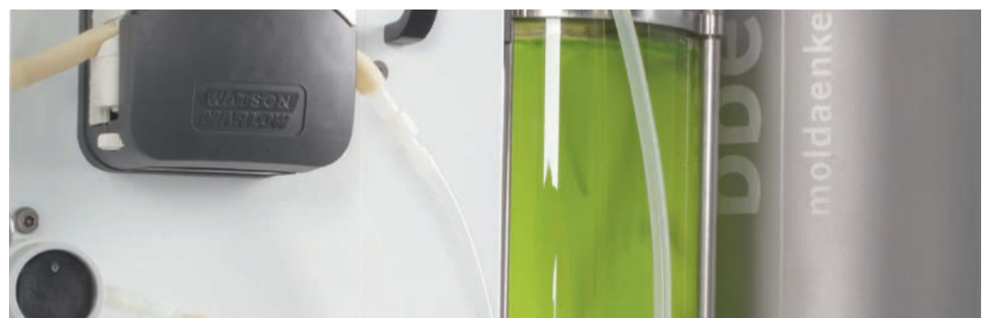
Sample water is mixed with the algae test solution and then analyzed
