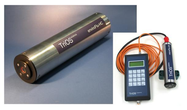
The enviroFlu-HC miniature fluorometer allows the user to monitor online polycyclic aromatic hydrocarbons (PAHs) concentrations by directly measuring the amount of fluorescence emission from a given sample volume. PAH's are excited by a high efficiency Xenon flashlamp. The required wavelength for PAHs excitation is selected by the use of an interference filter centred at 254nm.
