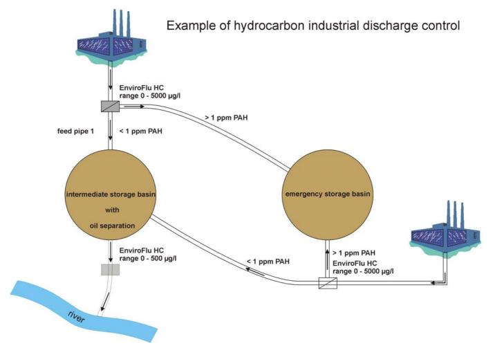
Renault car production in Fleine (France) is based on two sites. Surface water run off from both sites must be monitored and controlled for various parameters including Hydrocarbons. Monitoring stations are located as shown, two used for diverting flow to an emergency containment and one for monitoring final discharge to water course. Photographs of the installations are shown overleaf.
